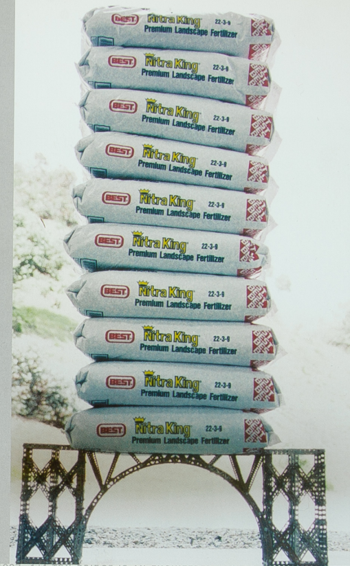
1/4 TON BRIDGE, 1997. 1/4 TON BRIDGE IS AN ENGINEERED ARCH BRIDGE CONSTRUCTED OF MECCANO AND ERECTOR PARTS. IT IS CAPABLE OF SUPPORTING 500 POUNDS. THE THIN DIAGONAL STRUTS ATTACHING THE DECK TO THE ARCH ACTUALLY TRANFER THE CONSIDERABLE LOAD TO THE ARCH AND PREVENTS THE SPAN FROM COLLAPSING, SHOWN HERE LOADED WITH TEN 50 POUND BAGS OF FERTILIZER.
